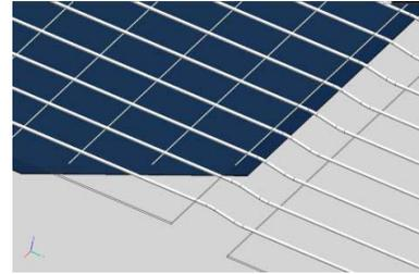
**Figure 13:** Close-up on flip-flop interconnection directly from one cell front surface to the next cell back surface.
