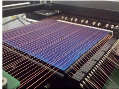
**Figure 4:** Full square  $156 \times 156 \text{ mm}^2$  SHJ cell produced by CIC measured using GridTouch<sup>®</sup> contacting technology developed by the company PASAN.
