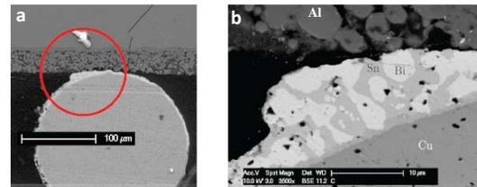
**Figure 14:** SEM image of the cross-section of the BiSn coated copper wire in contact to Al BSF. The BiSn coating microstructure is evidenced in the right image, with almost pure Bi phase and Sn phase with up to 20 %wt Bi.
