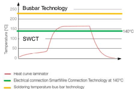
**Figure 3:** Temperature for connection with busbar technology, with SWCT as well as for module lamination.
