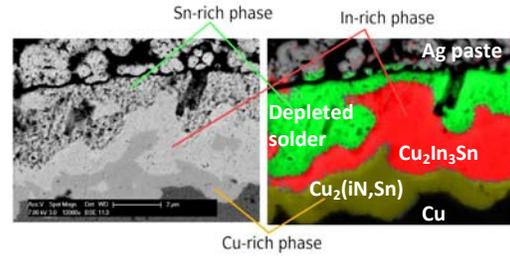
**Figure 10:** SEM-BSE image of the wires outer layer different phases. Wire coated contacted to low temperature silver paste (visible in the upper part of the image).
