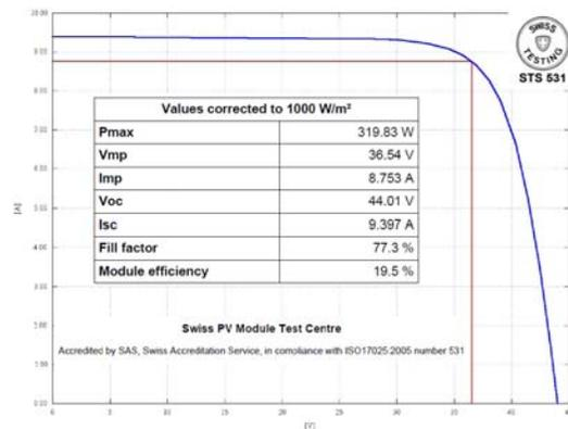
**Figure 5:** Certified IV curve of Gen2 module based on full square CIC SHJ cells and SmartWire Contacting Technology (SWCT). Certification was done by SUPSI Swiss PV Module Test Centre.
