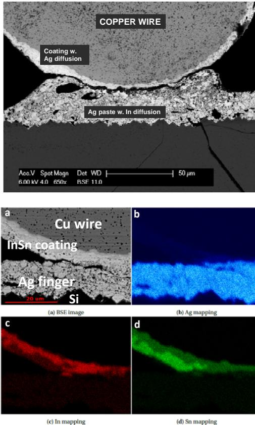
**Figure 9:** (a) Back scattered scanning electron microscopy (SEM) image and (b-d) energy dispersive x-ray spectroscopy (EDX) mapping of the contact between
