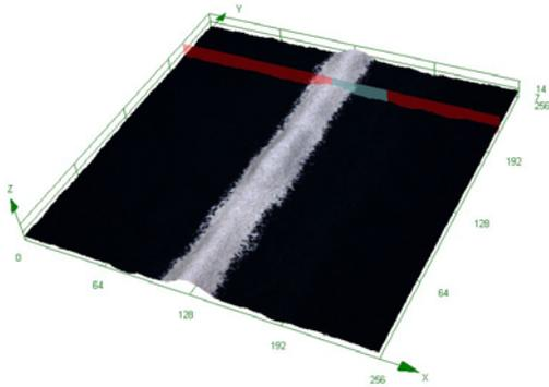
**Figure 15:** 3D reconstruction using a laser scanning confocal microscope (Olympus LEXT) of a low temperature silver paste printed with a 20  $\mu\text{m}$  screen opening.
