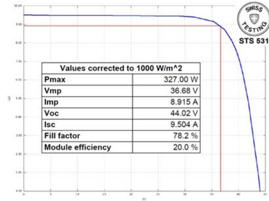
**Figure 6:** Certified IV curve of Gen3 module based on full square CIC SHJ cells and SmartWire Contacting Technology (SWCT). Certification was done by SUPSI Swiss PV Module Test Centre.
