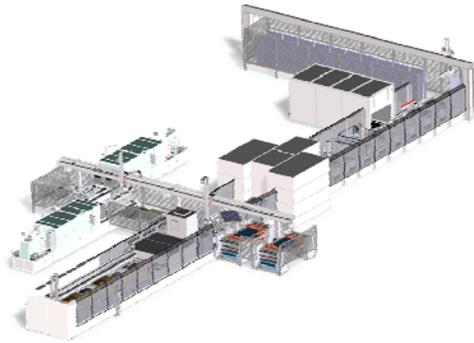
**Figure 11:** SWCT-GG module line with a 90 MW production capacity.
